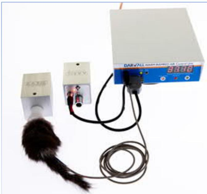
**Figure 4** Shows 2 ZDS Qube. The ZDS Qube block on left shows rodent in a mask being monitored by an auxiliary temperature probe. The ZDS Qube block in the centre is connected to the Heated Breathing Circuit controller which provides power and monitors the temperature of the block. The HBC control is on the right.
