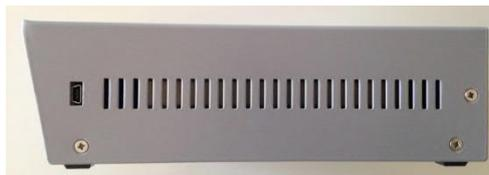
Figure 7 HBC right hand side view (note USB port)
